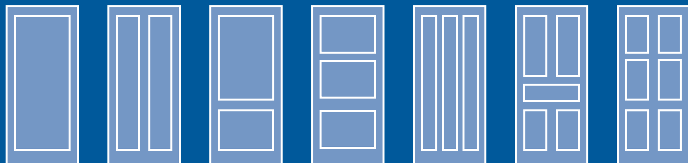
1 PANEL 2 PANEL 2 PANEL 3 PANEL 3 PANEL 5 PANEL 6 PANEL
